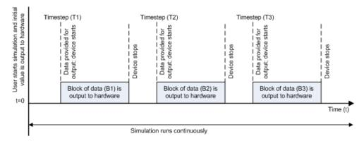
Scenario 1 shows the case when data output speed outpaces simulation speed. At the first time step (T1), data output is initiated and the corresponding block of data (B1) is output to the hardware. The simulation runs continuously in this mode.
