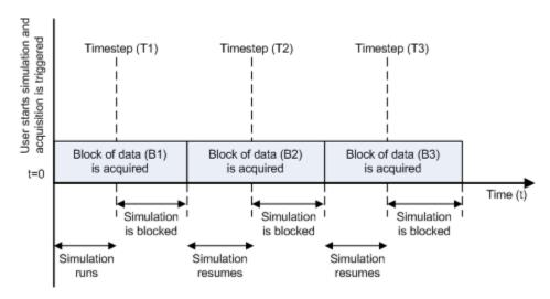
Scenario 1 shows the case when simulation speed outpaces data acquisition speed. At the first time step (T1), the required block of data (B1) is still being acquired. Therefore, the simulation does not continue until B1 is completely acquired.
