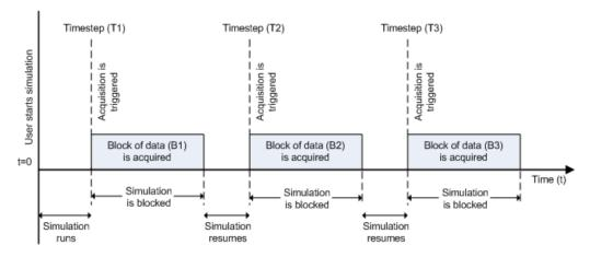
At the first time step (T1), the acquisition is initiated for the required block of data (B1). The simulation does not continue until B1 is completely acquired.
